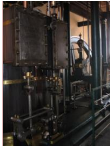
Figure 4.90: The valve gear chests with the worn valve gear rods.
