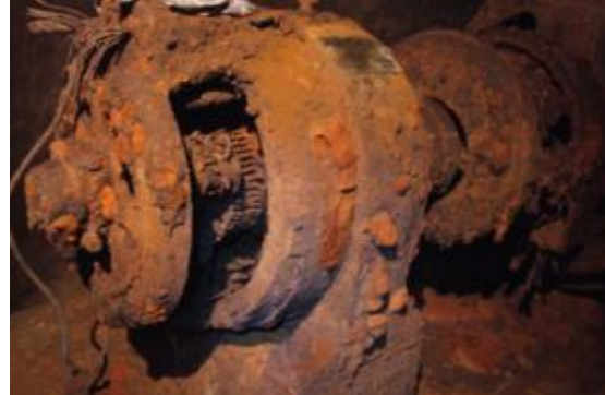
Figure 4.105: Crompton Motors with severe active rust.
